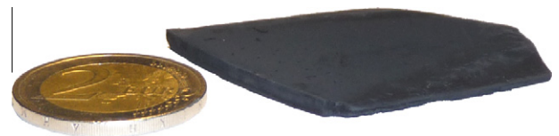
Fig. 2. Typical dimensions of as-grown product used for the production of the nanocomposite mats.
